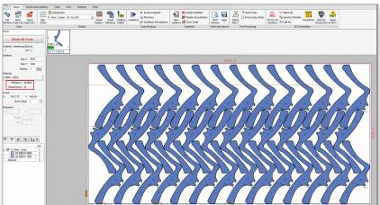
• A longer run of 300 seconds managed to fit 48 parts on the sheet.
