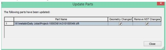
After changing the part dimensions, the SubNest changes (to the two MicroJoints) are not kept:
