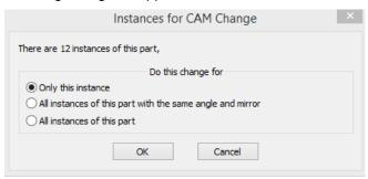
Determine if this change will be applied only to the current instance of the part, only to instances with the same angle and mirror, or to all instances.
