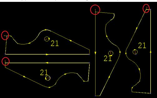
After you run **Smart Cut** with the **Top Left** corner option, **AutoNest** positions all the entry points at the top left corner, regardless of the part's orientation:
